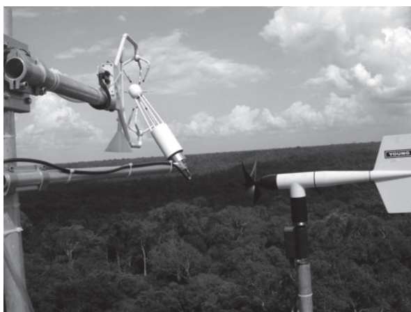
Figure 1: Our setup in operation: Wind Sonic, Licor, Young and methane analyzer inlet
